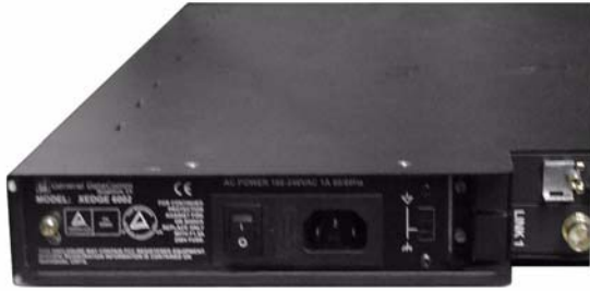
Partial view of chassis rear panel showing AC power connections.
