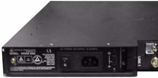
Partial view of chassis rear panel showing AC power connections. (Internal power supply not user accessible.)
