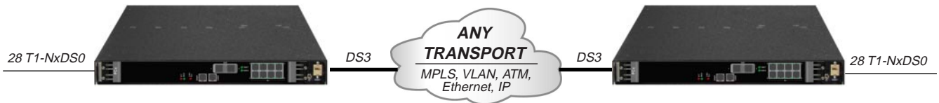
Figure 4 Channelized STM-1 with NxDS0
