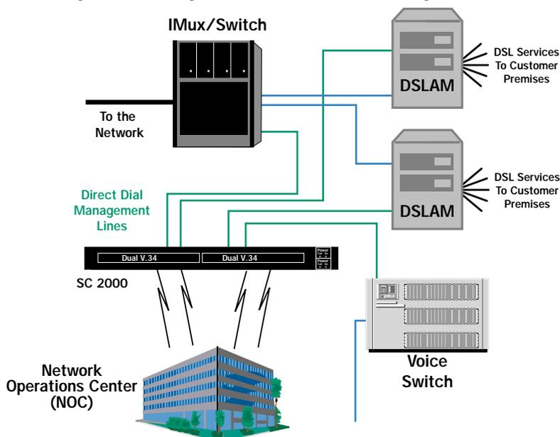
FIGURE 1 – ONE MANAGEMENT SERIAL PORT PER DEVICE
