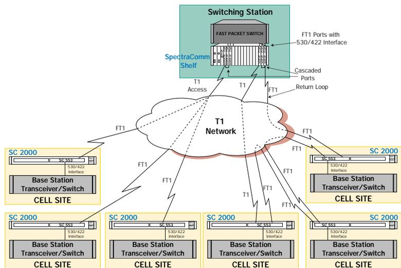
Figure 9 — T1 Access and Cascading Cell Site
