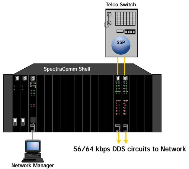
Figure 6 — Line-by-Line 56/64K Circuit
